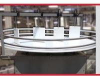
**Rotary Accumulation Table System.** Rotary accumulation tables provide a simple efficient method to provide a buffer for accumulation for downstream operations or at the end of the line for hand packing products. They are simple in design, come in various sizes to match the application and do not require any sophisticated controls.
