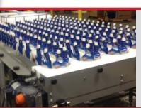
**Serpentine Accumulation System**. This accumulation system is an inline FIFO type system. These tables work well for both round containers and non-round containers. The line speed is set such that under normal operating conditions product is spaced on the conveyor as it transverses back and forth through the system. When downstream products stoppage occurs, the products accumulate by closing the gaps. These systems provide increased inline accumulation in a compact footprint.
