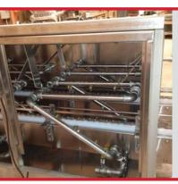
**Full Can Water Rinsing Systems.** Simple yet effective way to clean the full cans upon leaving the closing operation. Stainless steel enclosures with powered thru conveyor or gravity track. Multiple spray bars and spray nozzles for rinsing the containers as they pass thru.
