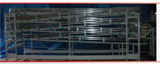
Cable Alpine System. A cable alpine system is ideal for many applications requiring accumulation, storage or elevation change. A cable alpine system takes up minimal floor space and is a simple way to provide inline accumulation. Cable conveyor systems are great for conveying and accumulating light weight empty containers.
